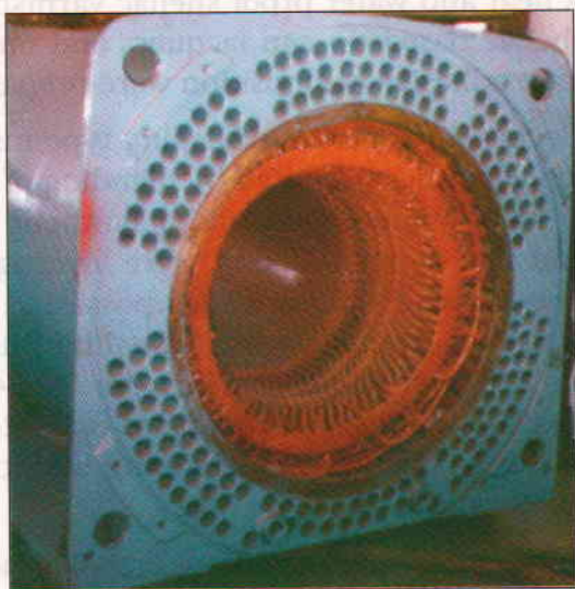
Electric motor applied with shellac-based insulating varnish
