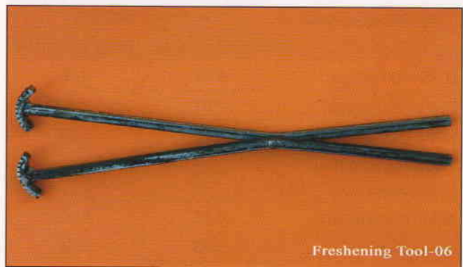
Fig. 87 View of scissor and blade type freshening tool
