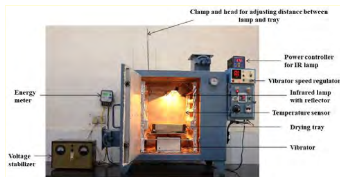
Fig. 3.20b: Interior view of IR dryer
