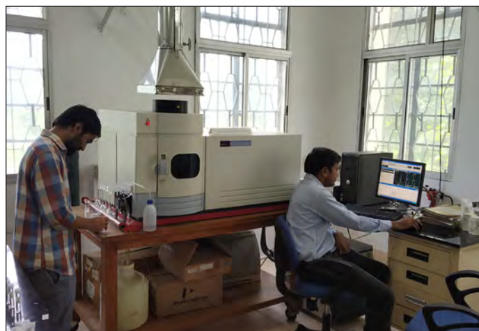
Fig. 4.14a: Analysis of water sample by ICP-OES
