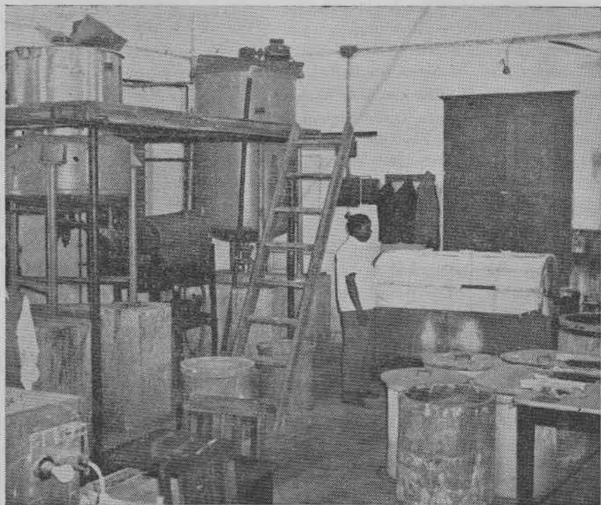
Bleached lac pilot plant
